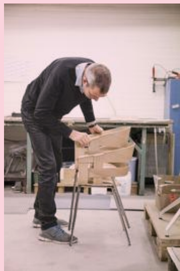
Designer Karl Malmvall testing the chair's stackability at the factory in Nybro, Sweden. 3D printed models of various options for support to the left.
