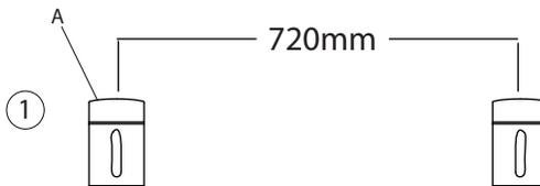
Mount the brackets on the wall with 720mm from center to center
