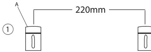
Mount the brackets on the wall with 220mm from center to center
