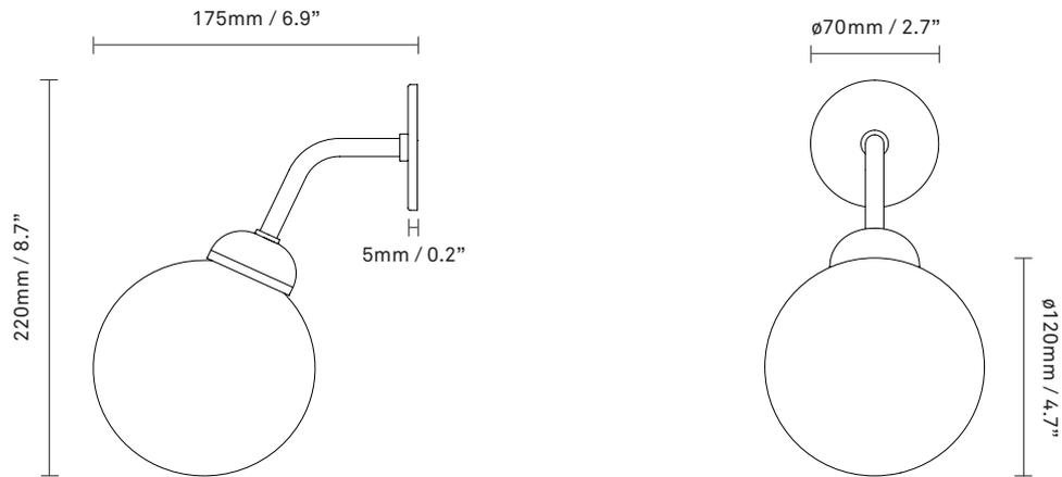
**Apiales Wall Hard-Wired** is connected directly to the electrical wiring in the wall. A classic wall plate version of the Apiales Wall lamp is also available.
