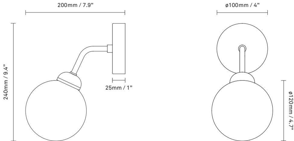
**Apiales Wall** is available with a classic wall plate or as a hard-wired version, to be connected directly to the electrical wiring in the wall. Wall plate fits US 3½" pancake bracket.
