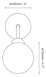
**Apiales Wall** is available with a classic wall plate or as a hard-wired version, to be connected directly to the electrical wiring in the wall. Wall plate fits US 3½" pancake bracket.
